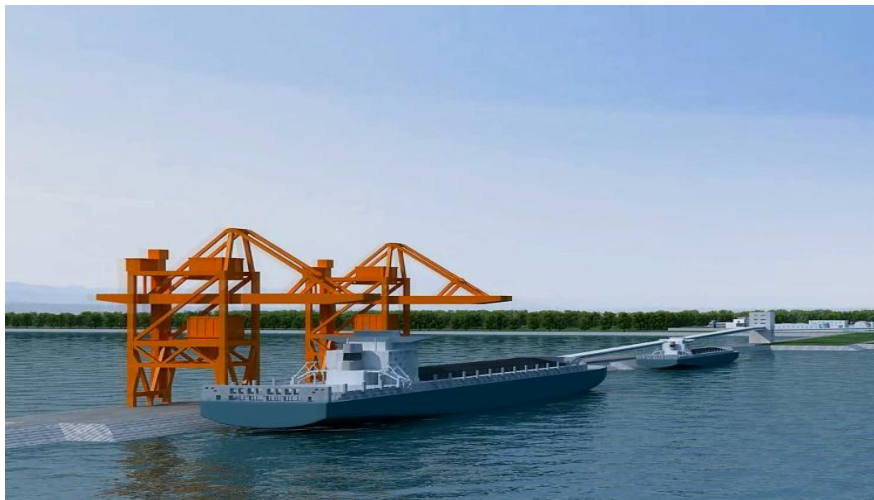
Figure 3-4 An Artist illustration of the Bridge Type Grab Unloader and Belt Conveyor Arrangement
