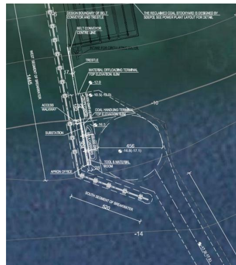
Figure 4-4 Plan II of Belt Conveyor Trestle
